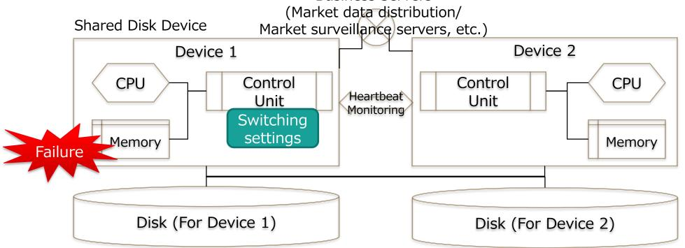
\*In tests before go-live, we turned off heartbeat monitoring between Device 1 and Device 2 and confirmed that automatic switching occurred swiftly.
